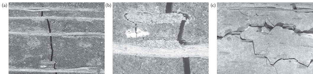
FIGURE 13.18 Crack propagation in pultruded glass textile composite: (a and b) crack propagation across the loading direction shown by arrows and (c) cracking across and along the loading direction at failure.
