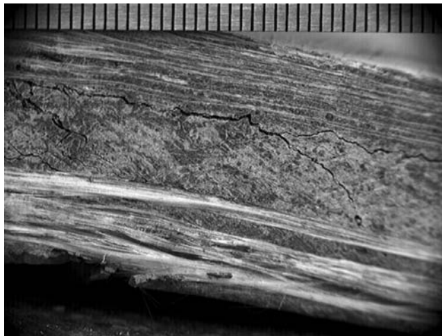
FIGURE 10.11 Ply delamination cracking in a flexural specimen (scale markers = 1 mm).
